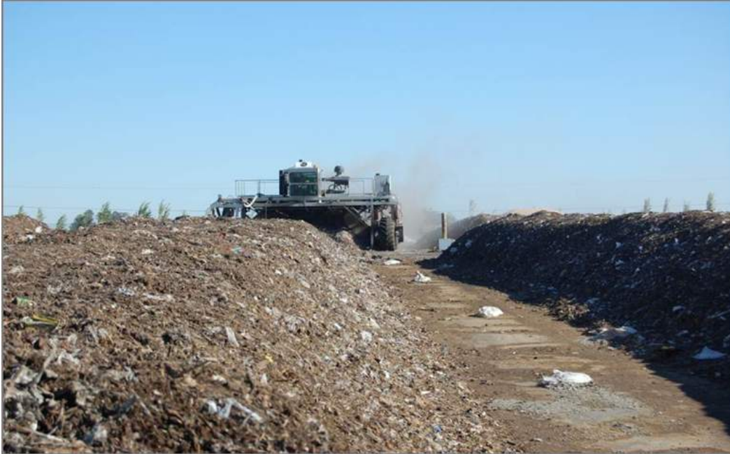
Figure 8: Example of a Windrow Aerobic Composting Facility
