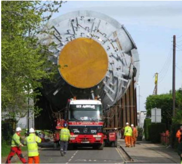
Figure 6: Alter NRG 1,000-TPD Plasma Gasification Reactor Tees Valley, England, UK
